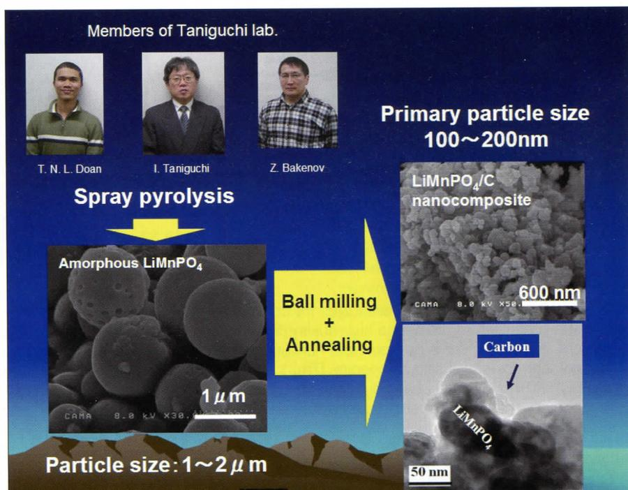
that were usable with their lithium-ion battery prototype. By adopting the resultant electrode into the battery, a voltage of approximately 4.1V was achieved in addition to the marking of a high percentage of energy output, ninth-tenths of the theoretical maximum output.
